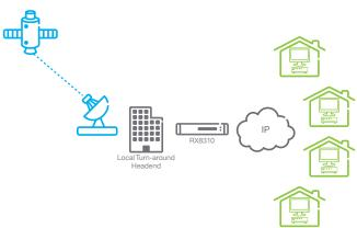
The RX8310 offers capability to descramble single or multiple services outputting the descrambled transport stream into the local station either as ASI or IP. Using the RX8310's multi-format capability the receiver can decode any 4:2:0 SD or HD MPEG-2 or MPEG-4 service to analog SD to interface into a legacy analog tier or for local monitoring.
